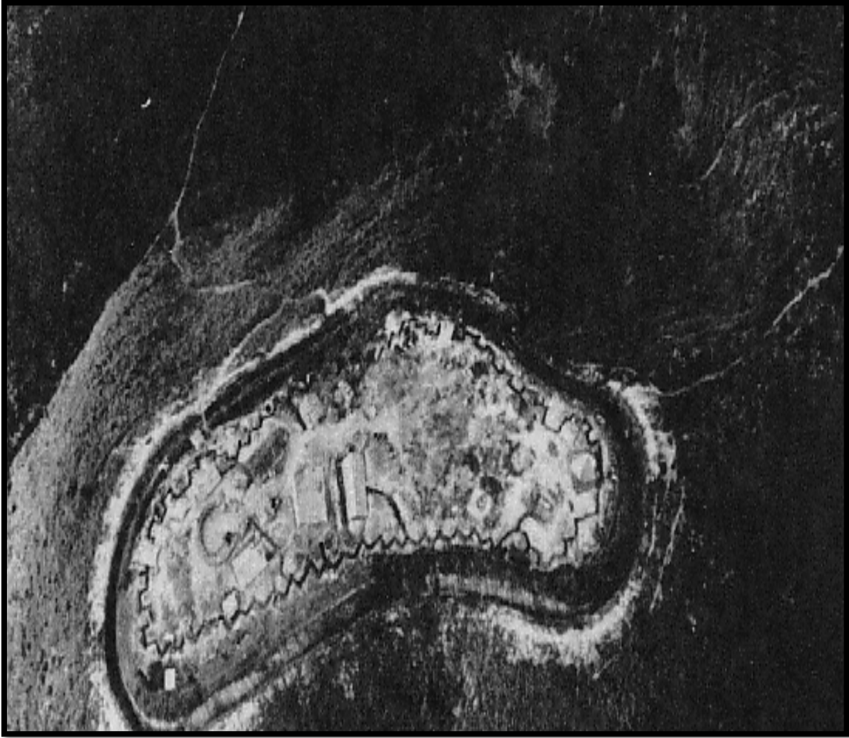
Overhead view of a kidney shaped mountaintop Meo defensive fighting position at Bouam Long. Note the zigzag shaped trench system that afforded additional field of fire.
