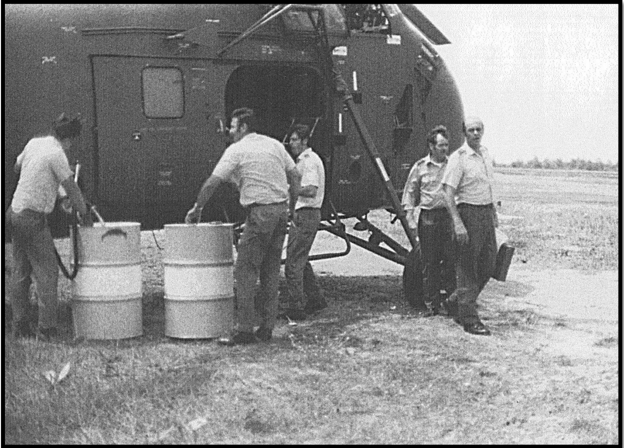
Manual refueling with wobble pumps from drums at Hua Hin, Thailand on the ferry trip down the western peninsula to Jakarta, Indonesia. Air America Personnel left to right: Steve Sickler, Gaza Eiler, Emmet Sullivan, Duane Keele, and Hal Miller.
