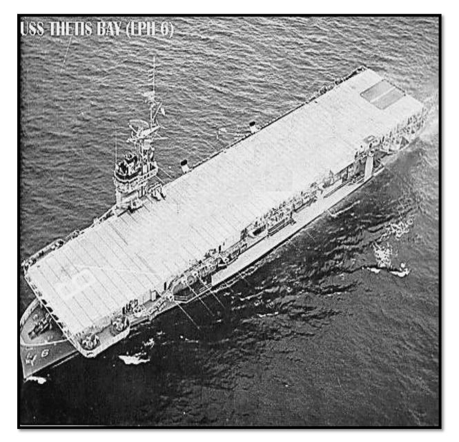
USS *Thetis Bay* carrier without a visible complement of Marines and helicopters. A single elevator is at the stern of the ship. Author Collection.
