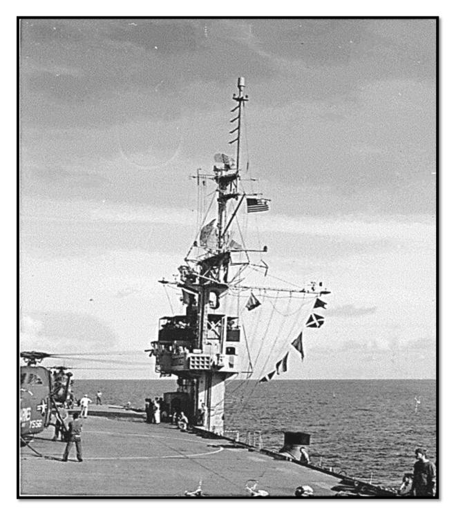
USS Thetis  $Bay^\prime s$  infamous superstructure that caused a noticeable starboard list of up to eleven degrees.
