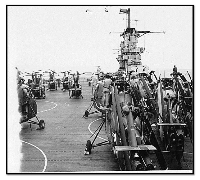
USS *Princeton* flight deck. To the right, HUS-1 blades and tail pylons remain folded after being raised on elevators from the hanger deck prior to flight operations. Kaman HOK aircraft are seen parked forward. One HUS-1 is departing from spot one on the ship's bow.
