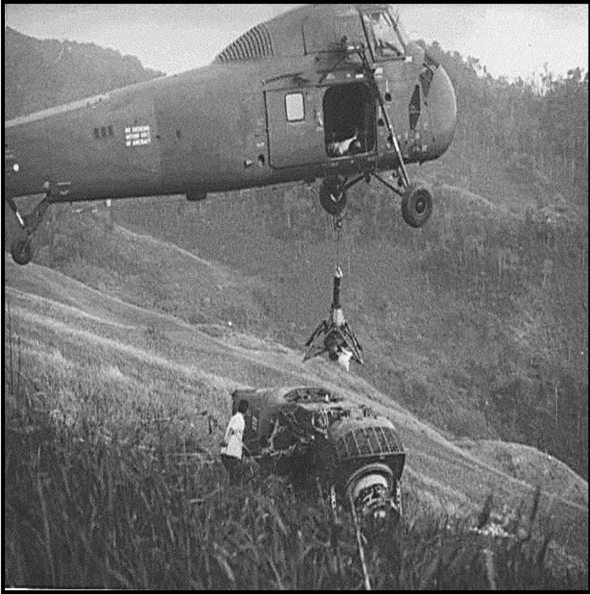
Removal of the transmission without the rotor head to Sam Tong. Straps and cables are strung and secured upslope to prevent the helicopter from rolling downhill from effects of the helicopter downwash.
